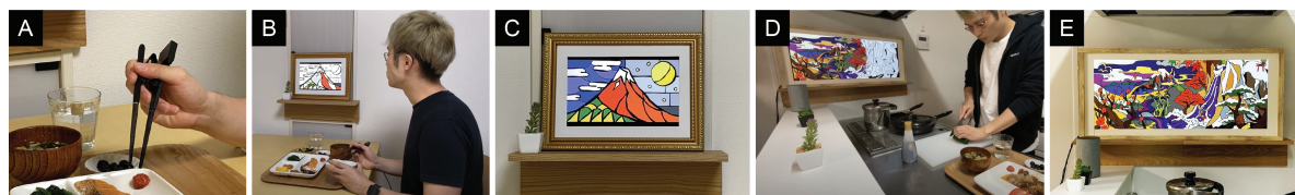
Fig. 1. By transforming eating into a task of progressively coloring a landscape projected onto a screen, the eat2pic system encourages users to eat more slowly and maintain a healthy balanced diet. The eat2pic system is composed of a calm sensing component based on a sensor-equipped chopstick (A) and visual feedback components using two types of digital canvases (C, E). The colors of the foods consumed by the user are shown on one part of a landscape displayed on two digital canvases to illustrate a single meal and the food consumed in a week as digital paintings generated by an automated system. The one-meal eat2pic (B, C) guides a user's behavior through a single meal with real-time feedback, whereas the one-week eat2pic (D, E) guides a user's food choices and eating behaviors with longer-term feedback accumulated over a full week.
